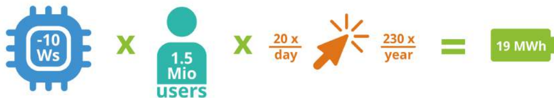
Figure 11: One CPU-second reduction is roughly equivalent to 10 watt-second savings. If 1.5 million users use the software, and there are 20 transactions a day with the savings over 230 work days, that is about 19 megawatt-hours savings. (Image from KDE published under a CC-BY-SA-4.0 license. CPU icon by Azland Studio and Cursor icon by Alice-vector licensed under a CC-BY license. Design by Lana Lutz.)
