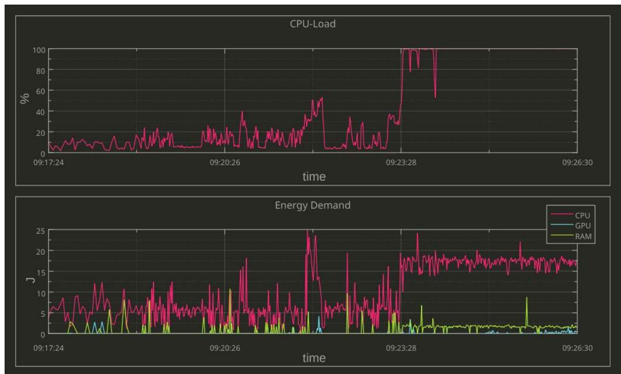
Figure 19: Monitoring energy and hardware consumption in real time with KDE’s LabPlot. (Image from Alexander Semke published under a CC-BY-NC-ND-4.0 license.)
